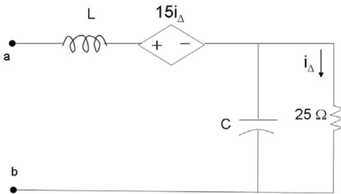
Find the input impedance  $Z_i$  at the terminals a,b in the circuit shown above
