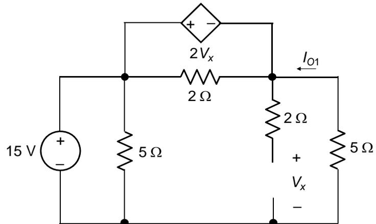
With  $V_{SRC2}$  applied and  $V_{SRC1}$  set to zero, the circuit becomes as shown. It follows that:  $-2V_x = V_x + \frac{2V_x}{jX_C}$ , or  $V_x \left( 3 + \frac{2}{jX_C} \right) = 0$ , which
