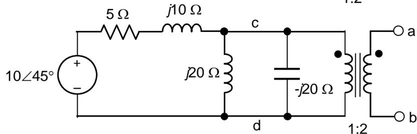
If the independent voltage source is replaced by a short circuit, the impedance on the primary side is  $(5 + j10) \Omega$  and  $Z_{Th} = 4(5 + j10) = 20 + j40 \Omega$ .
