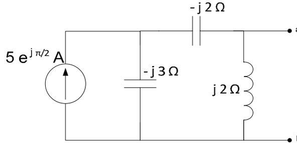
4. Find the Thevenin equivalent circuit with respect to the terminals a-b. What are the values of  $V_{Th}$  in V and  $Z_{Th}$  in  $\Omega$ ?
