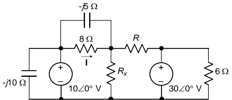
7. Determine the maximum power that can be delivered to  $R_L$ , assuming  $R = 0.5 \Omega$ .
