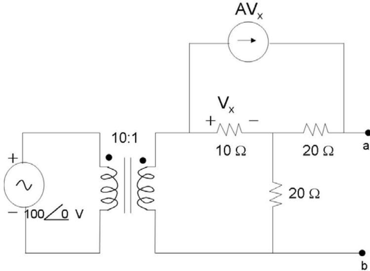
Find the magnitude of the Thevenin Voltage  $V_{th}$  across terminals a,b in the circuit above. Given  $A=1/4$ .
