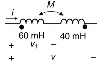
2. Determine  $\mathbf{V}_o$ , given that  $\mathbf{I} = 1 \angle 0^\circ \text{ A}$  and  $\omega = 10 \text{ rad/s}$ .
