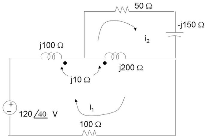
Given the circuit above, what are the two mesh equations?
