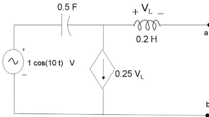
Find the Thevenin equivalent resistance and capacitance/inductance with respect to the terminals a,b in the circuit shown above
