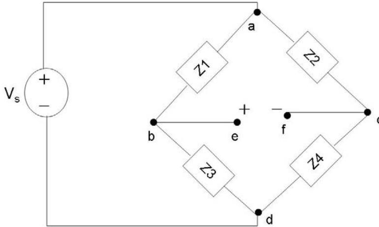
In the circuit shown above, given  $V_s = 48\angle 90^\circ$  V,  $Z_1 = 3 + j4 \Omega$ ,  $Z_2 = 8 - j6 \Omega$ ,  $Z_3 = 3 - j4 \Omega$  and  $Z_4 = 8 + j6 \Omega$ . The Thevenin equivalent circuit values for the voltage source and the internal impedance across terminals e and f are:
