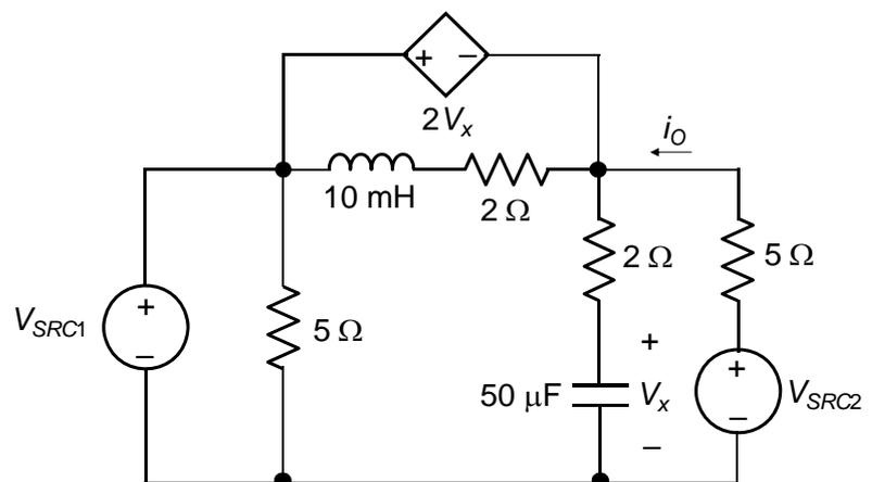
**Solution:** With  $V_{SRC1}$  applied and  $V_{SRC2}$  set to zero, the circuit becomes as shown.  $15 = 3V_x$ , so that  $V_x = 5$  V and  $I_{O1} = \frac{-V_x}{5} = -1$
