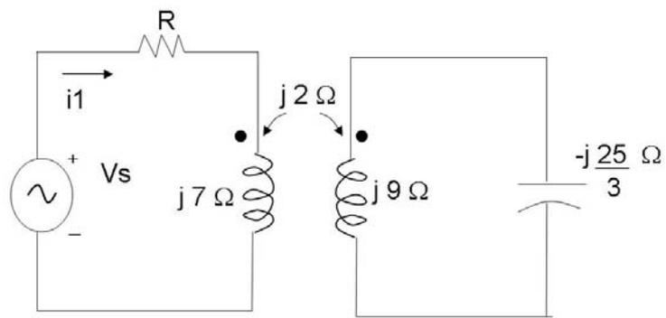
In the circuit shown above, it is given that  $R=1 \Omega$ , and  $V_s= 10\angle 0$  volts. Find the current  $i_1$  as indicated.
