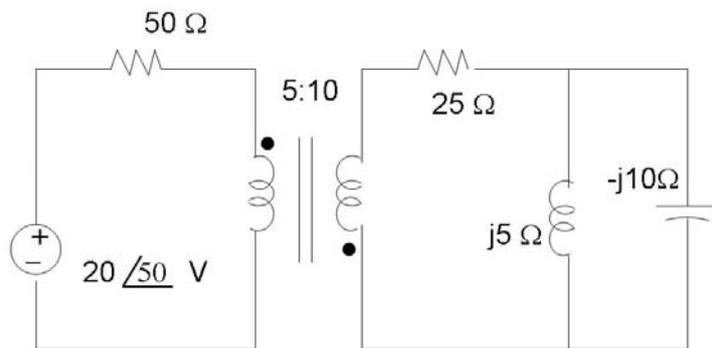
In the circuit shown above, what is the value of the reflected impedance of the 50 ohms resistor from the primary to the secondary side?
