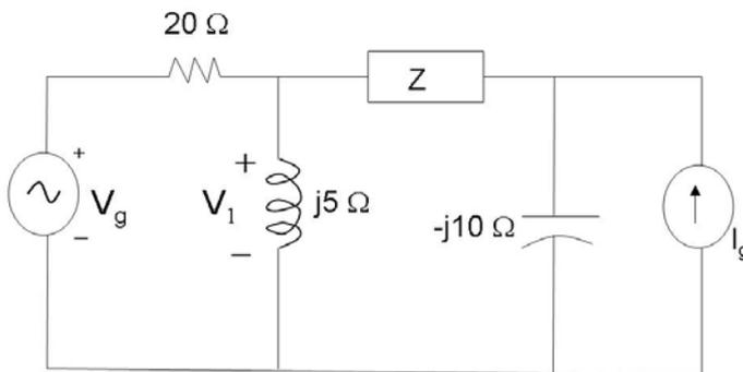
In the circuit shown above, find the value of the impedance  $Z$  if  $V_1 = 40 + j30 \text{ V}$ ,  $V_g = 100 - j50 \text{ V}$ , and  $I_g = 20 + j30 \text{ A}$
