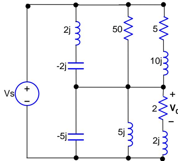
Find  $V_0$  if the source voltage is  $V_s = 20 \angle 60^\circ$  Volts.
