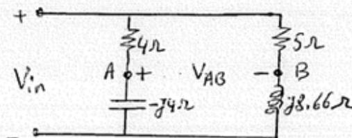
11. Considering the circuit below find its Thevenin impedance between a and b.
