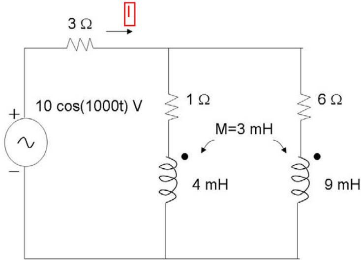
In the circuit shown above, the phasor form of the current  $I$  in amperes is:
