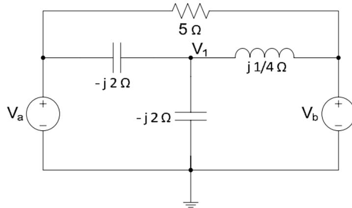
1. Find the correct node-equation for the voltage  $V_1$ .
